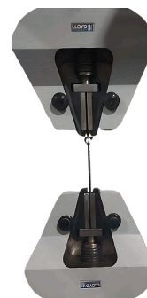
P2.5-20 - GUILLOTINE TRACTION BELT ( MAXIMUM TENSILE STRENGTH 12000 NW )
